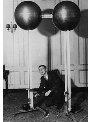
Figure 7. An early Van de Graaff generator being demonstrated by Robert J. Van de Graaff. [7]
